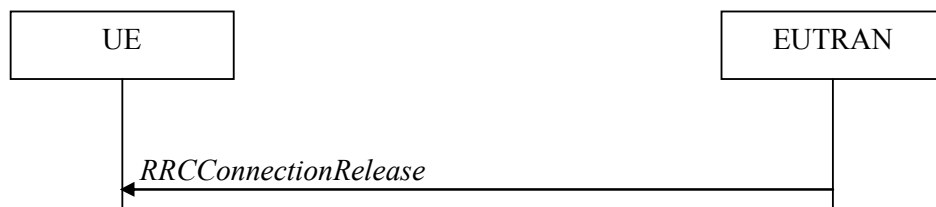
Figure 2: RRC connection release procedure [8]
