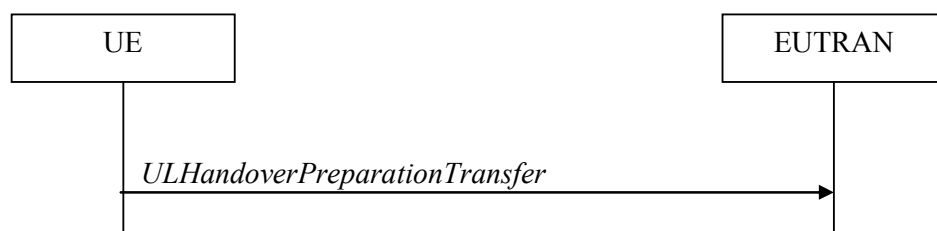
Figure 9: UL handover preparation transfer [8]
